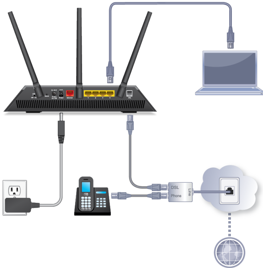
Figure 6. Modem router cabling for DSL service
