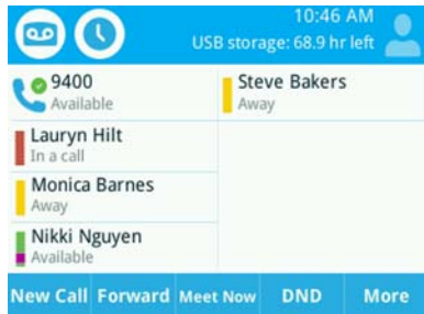
Figure 1: Favorite Skype for Business contacts on the Lines screen on VVX 500 series phones
