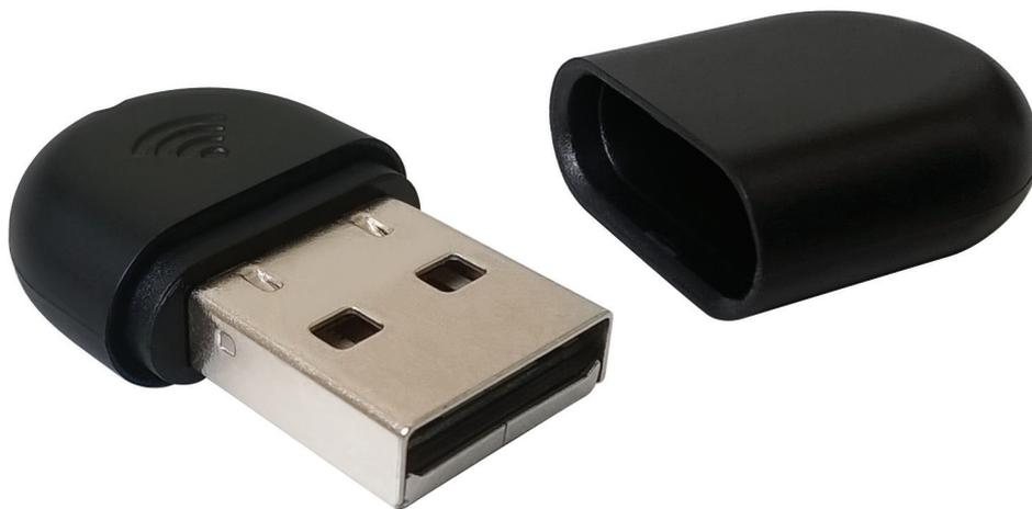
The WF40 Wi-Fi USB dongle is a low-power device that can be used to seamlessly connect the Yealink T48G IP phone to your organisation's wireless network. This dynamic plug-and-play USB device is an ideal office solution for companies seeking affordable and convenient connectivity.
