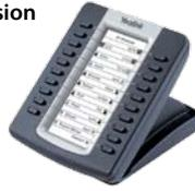
**EHS36 Electronic Hookswitch Adapter** Enables support for Plantronics, Jabra and Sennheiser DECT cordless headsets
