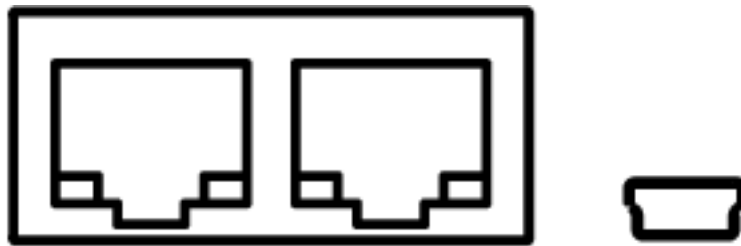
Figure 20: Network and USB Connectors
