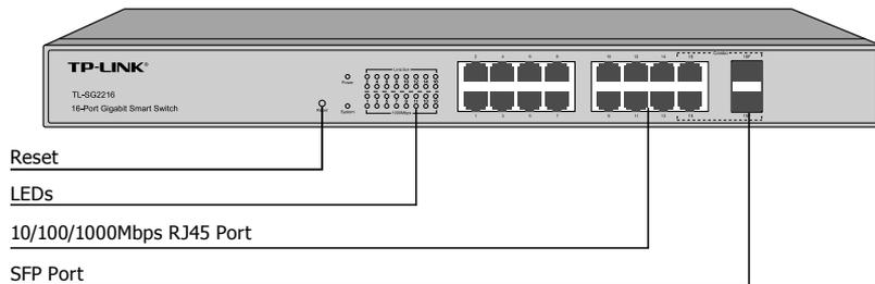
Figure 1-1 Front Panel of TL-SG2216
