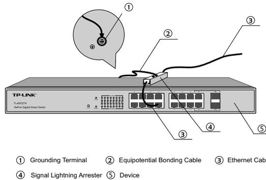
Figure 3-4 Lighting Arrester Connection
