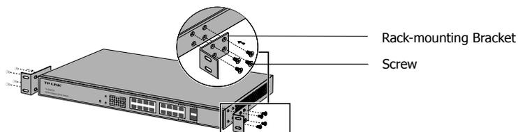
Figure 2-2 Bracket Installation
