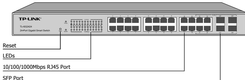
Figure 1-2 Front Panel of TL-SG2424
