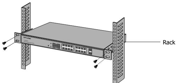
Figure 2-3 Rack Installation
