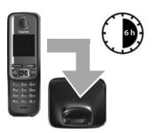
Charge the handset in the base station/charging cradle for 6 hours.
