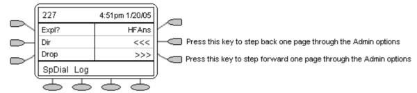
With the exception of **Expl?**, the names shown are the features that you can assign to soft keys. When **Admin** has been selected you can display the full name of the feature by pressing **Expl?**. See Longhand Programming Mode.
