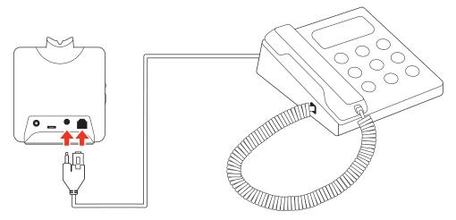
**Important:** Use configuration **A** on the back of the base, which works for most phones, including Cisco phones.
